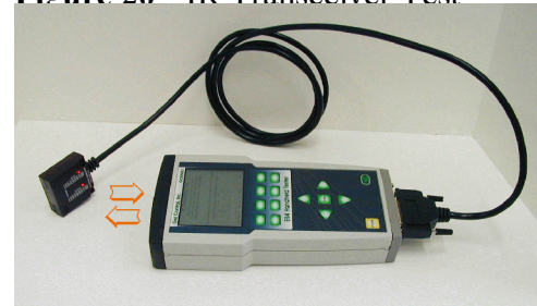
Figure 21 - IR Transceiver Test Alignment
